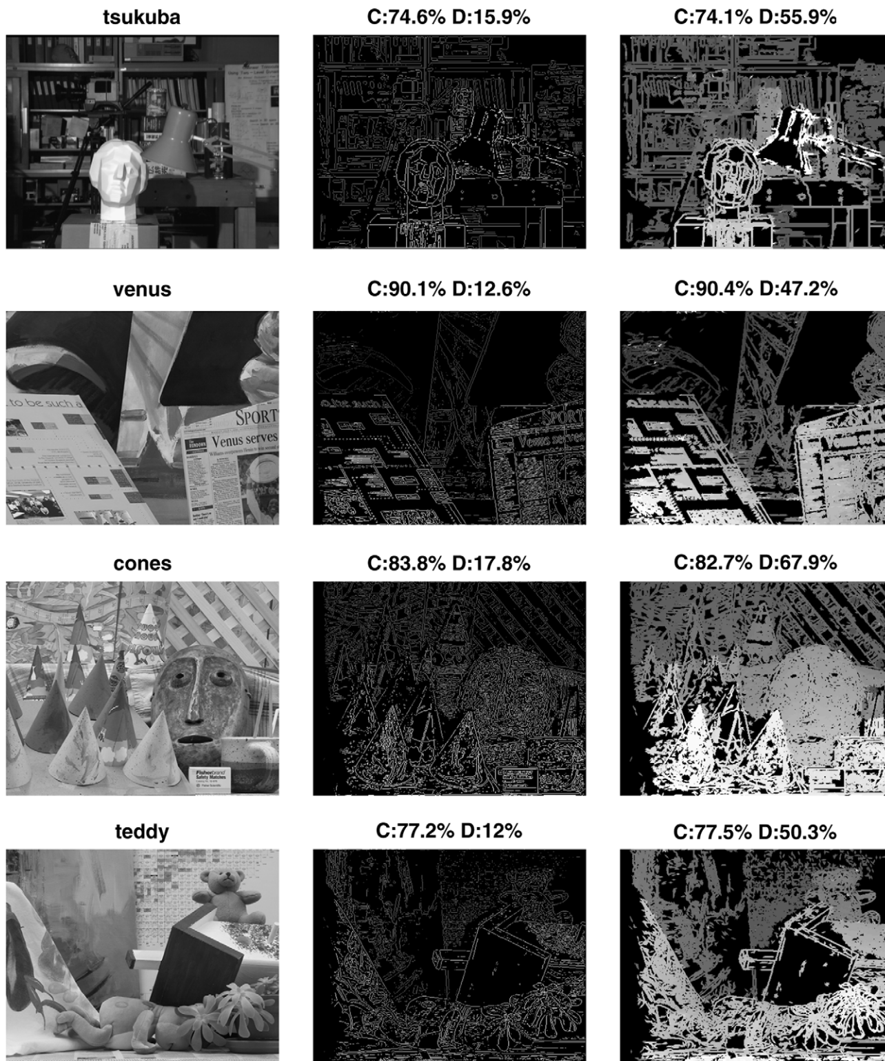
Fig. 2. Results for the test images: the left-hand column contains left-hand images of the original stereo-pairs, the middle column shows disparity maps calculated by dynamic programming and the right-hand column disparity maps densified using VMP. C denotes the percentage of correct disparities ( \pm 1 disparity level) and D, density.
